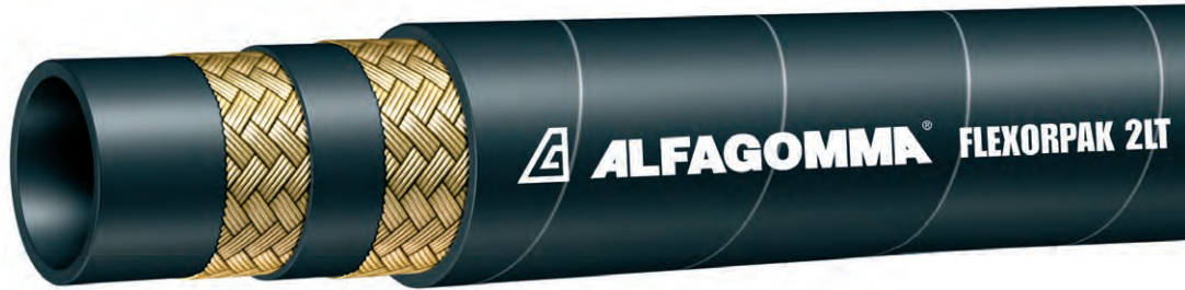
TF2LT – Double wire braid Meets or exceeds SAE 100 R16 - EN 857 2SC
