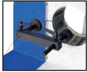
Back Limit Switch
