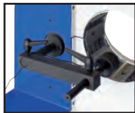
Back Limit Switch
